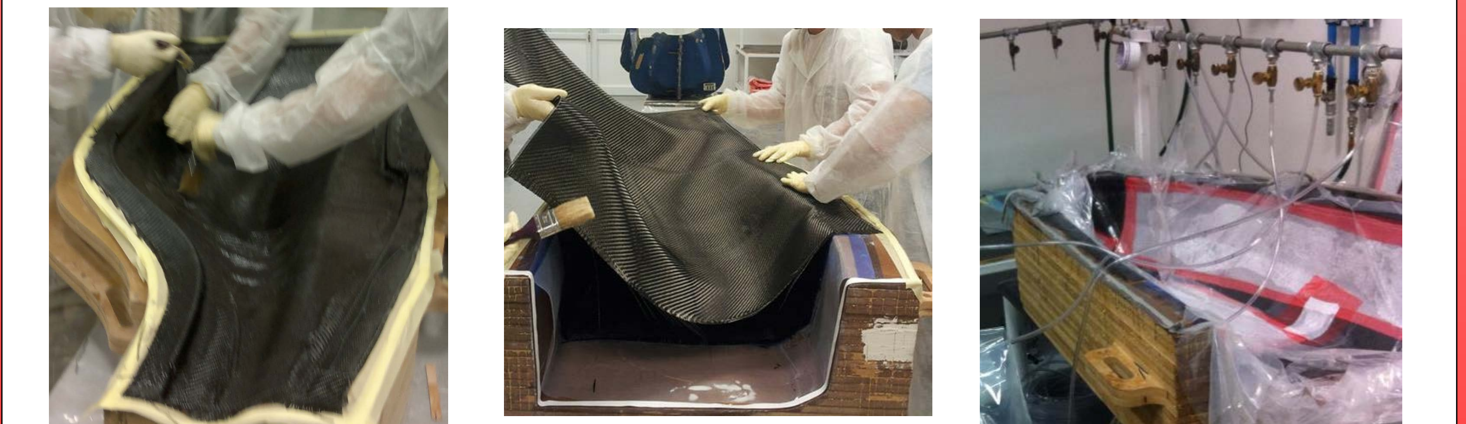
Figure 7: Layup and vacuum bagging the carbon fiber
