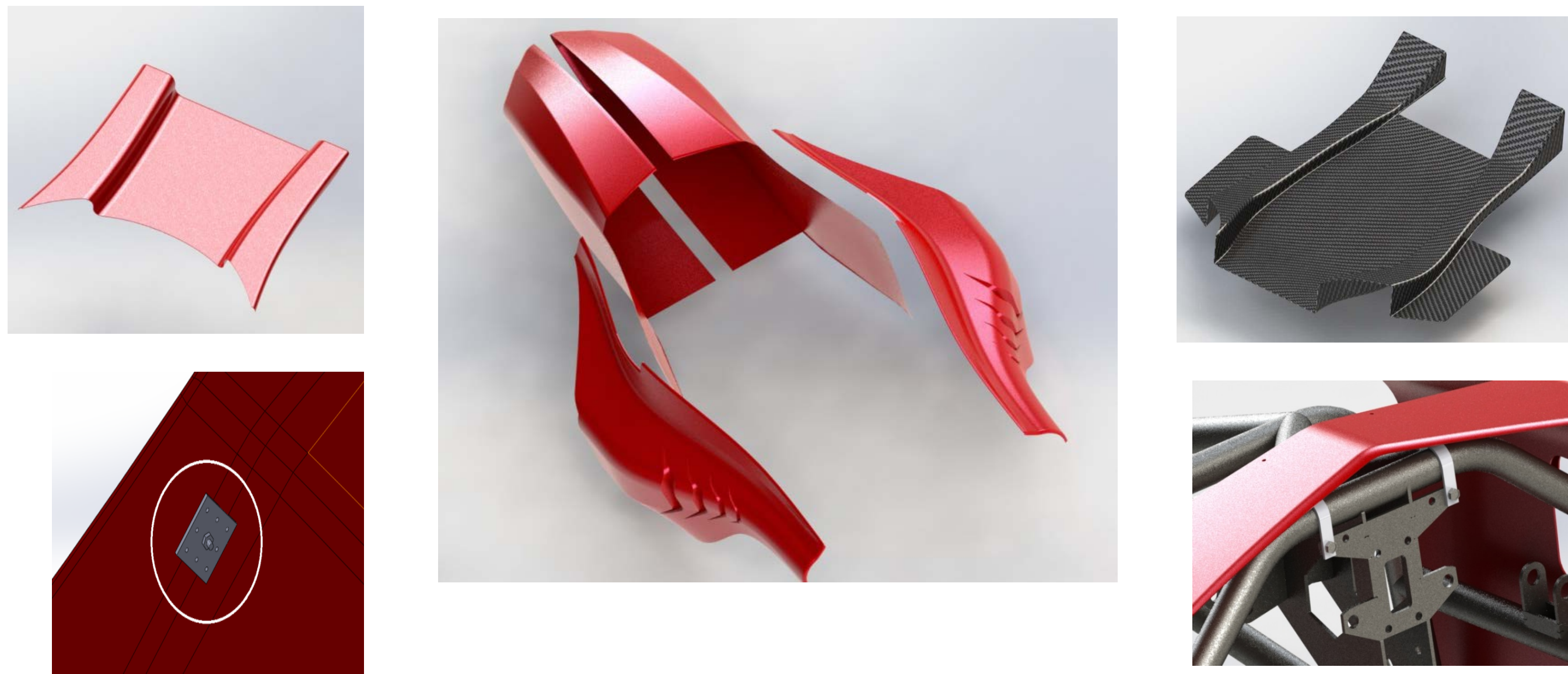
Figure 1: Segmentation and joining of the body parts
