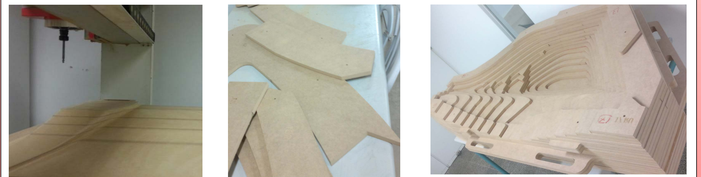
Figure 5: Machining & joining mold parts for the body
