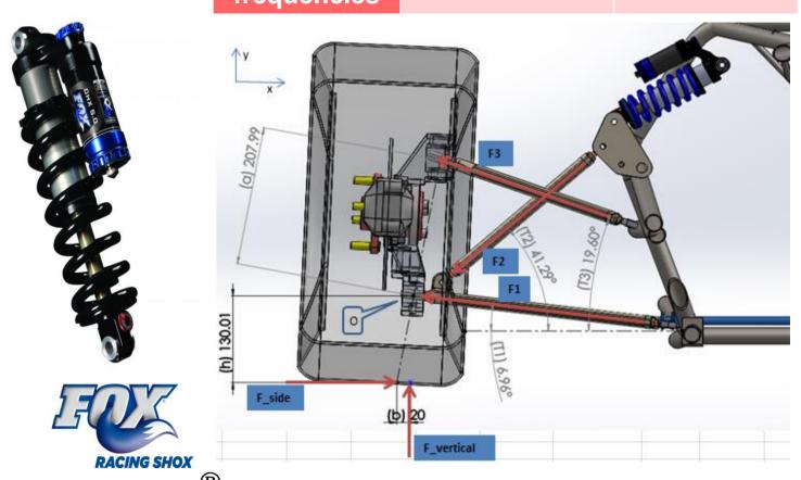
Finite elements analysis was performed using Solidworks® simulation tools to achieve the desirable factor of safety. A design study has been conducted in order to decrease weight while keeping the desired strength.
