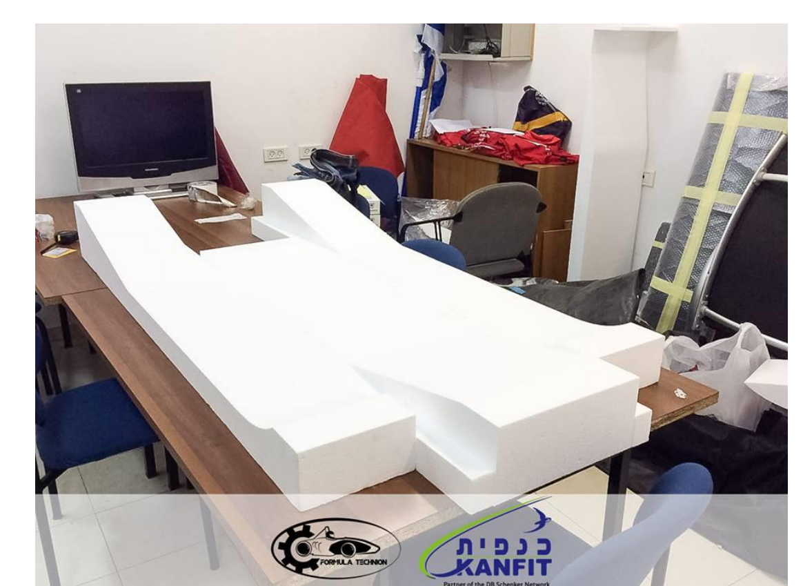
Undertray Mold - Styrofoam
