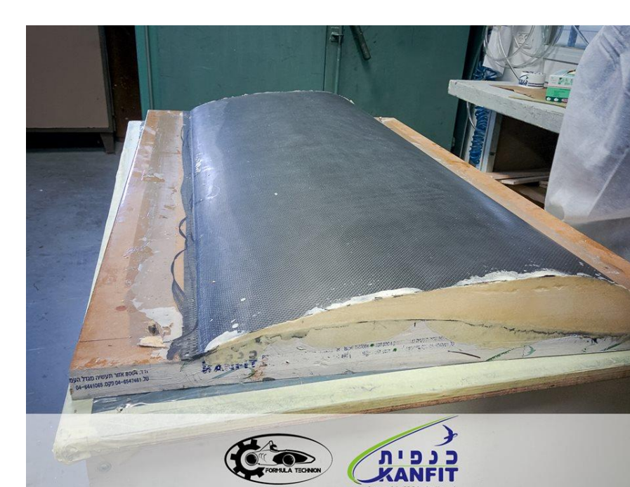
An airfoil filled with Polyurethane, for additional stiffness
