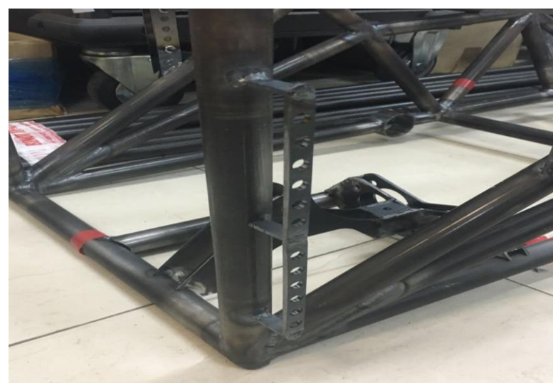
Steel bracket to mount the front wing
