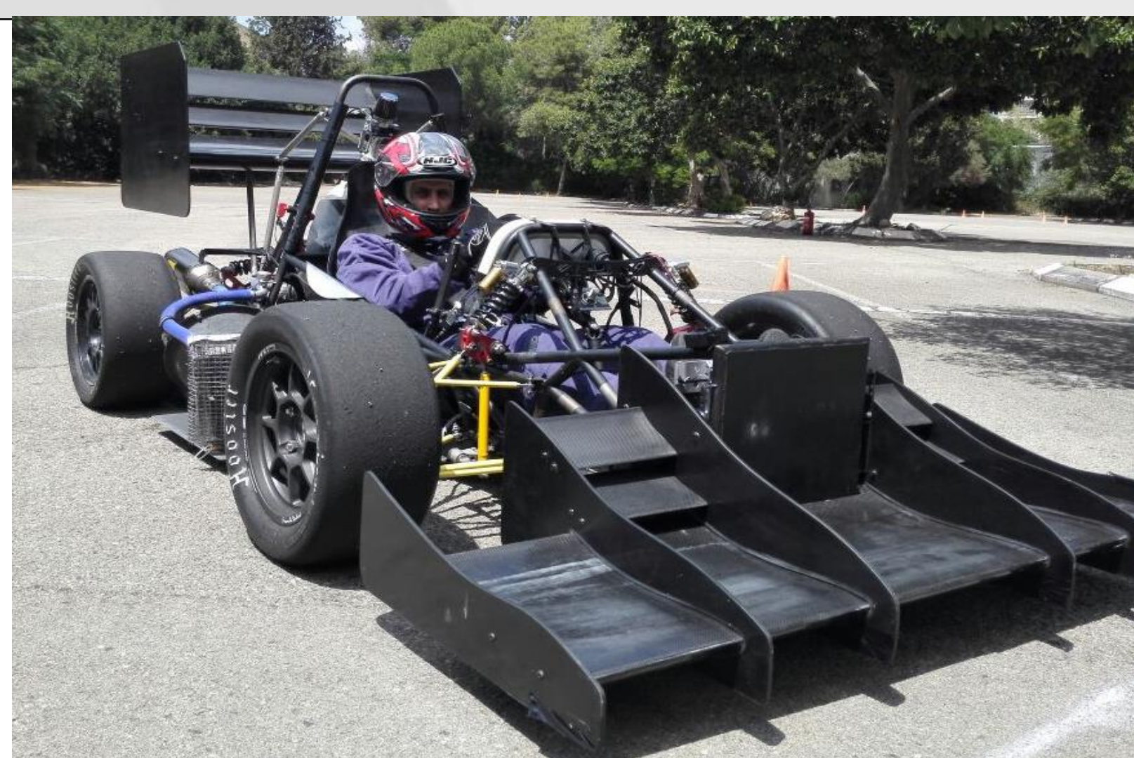
Undertray, Final product - Carbon With divinycell
