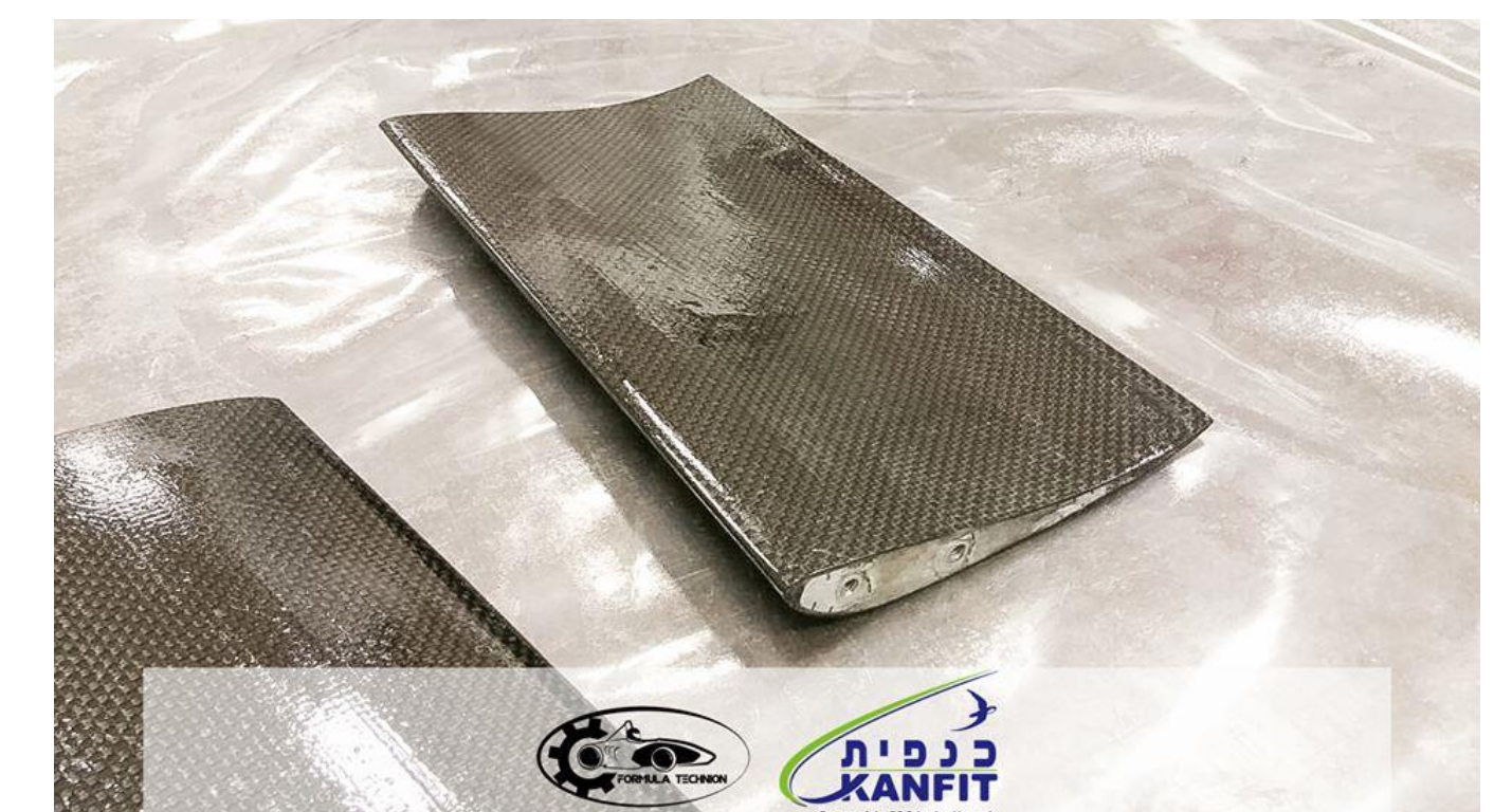
Full carbon airfoil filled with Polyurethane - With aluminum inserts
