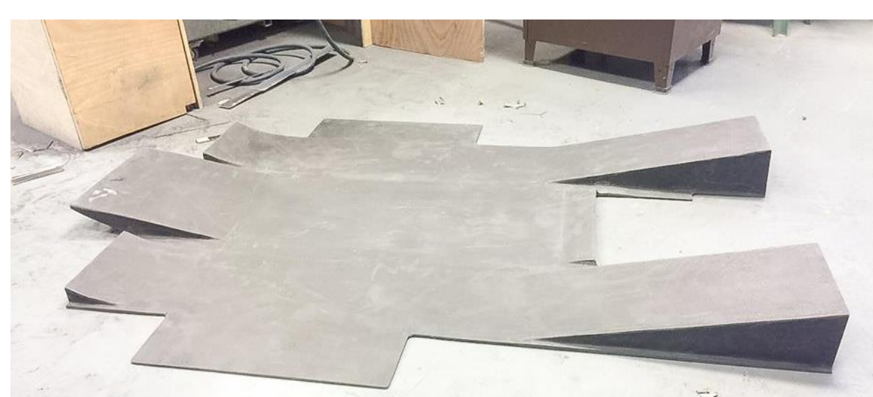
Undertray, Final product - Carbon With divinycell
